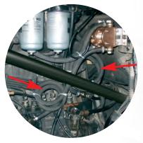
Example of an installation with increased length of hose connections
