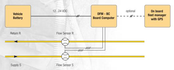
Connection of 2 single sensors (DFM8S, DFM20S, DFM25S) or of one double sensor (DFM8D) to the board computer.
