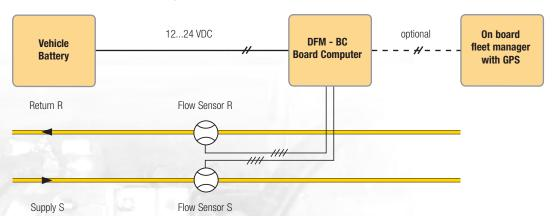
The board computer has a pulse output for the consumption that can be used as an input for a fleet manager or GPS system.
